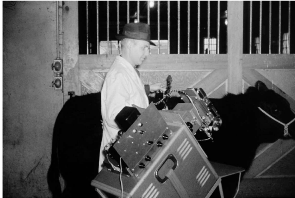
Figure 4. First scanner for the rib eye area with A-mode baseline recording using the Sperry Reflectoscope metal flaw detector equipped with the Polaroid camera and the mechanism to synchronize the transducer movement with the camera (Stouffer J.R. Author's personal collection).
