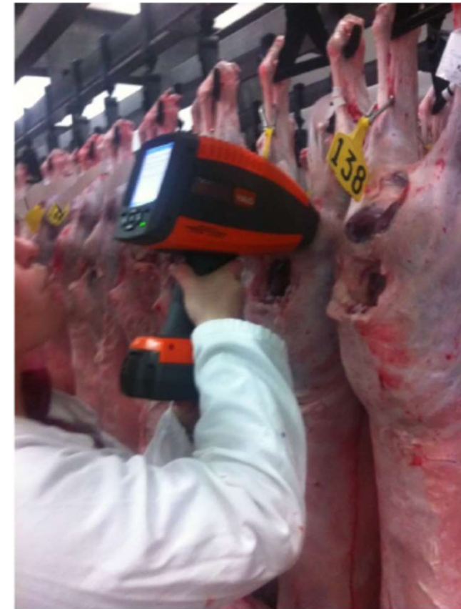
Fig. 1. Measurement of a lamb topside in-situ with a Halo® hand-held NIR device.
