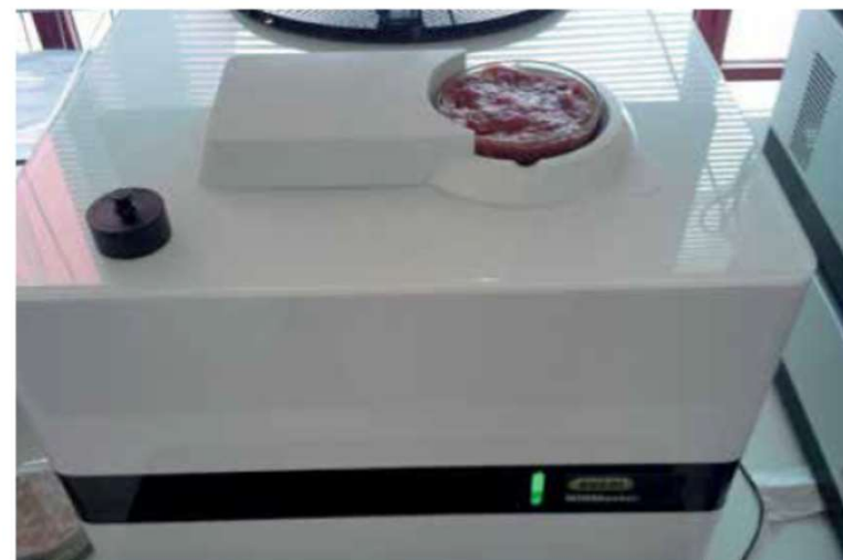
Figure 1. Process sample preparation and subsequent NIR Master analysis.
