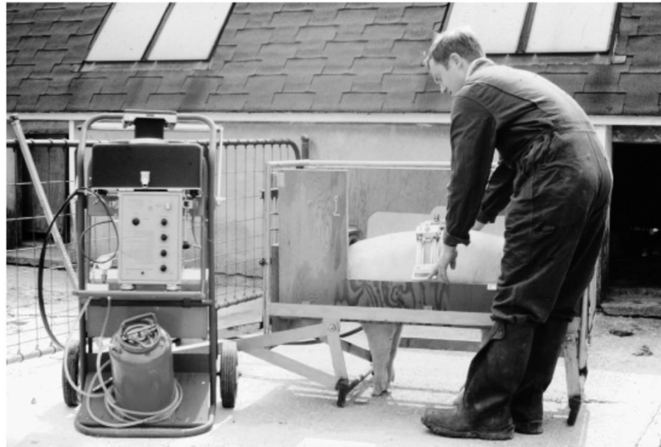
Figure 5. Scanogram, commercial mechanical B-scanner, model 721 produced by Ithaco Inc. being used for examination of a pig (Stouffer J.R. Author's personal collection).
