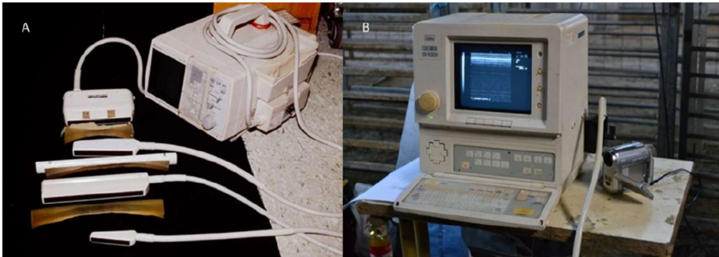
Figure 7. Aloka 210 scanner with several linear ultrasound probes and specially shaped standoff guides for each species (A) (Stouffer J.R. Author's personal collection) and Aloka SSD 500V equipped with a video camera to image capture (B) (Silva S.R. Author's personal collection).
