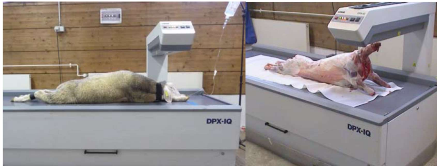
Figure 1: DXA scanning of a lamb in vivo and of a lamb carcass
