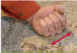
Brushing the back of the hand across the surface should not cause cuts
