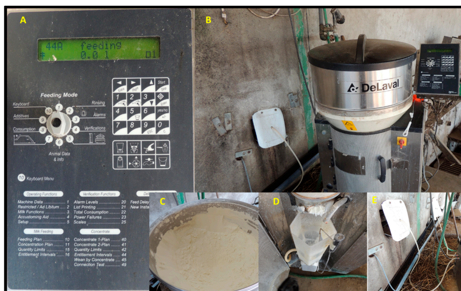
Figure 1. Automatic milk feeding system: (A) shows the control panel, where all the information relative to the calves and the machine is registered and controllable; (B) shows all the components (except the RFID reader and the teat, which are inside the calves' barn); in (C) shows the milk powder deposit; (D) is the mixer cup, where each portion of milk is prepared with milk powder and heated water; in (E) is shown the circuit in which the milk departs from the mixing cup to the teat inside the calves' barn.
