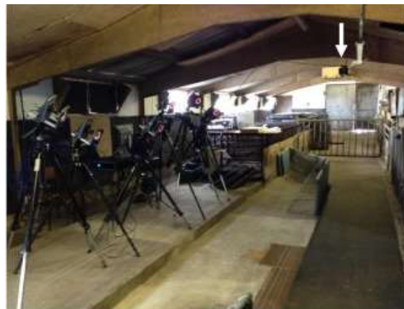
(A) Gait lab set-up showing the Vicon cameras with infrared strobe around each lens, and the Kinect camera mounted above the walkway (arrow).
